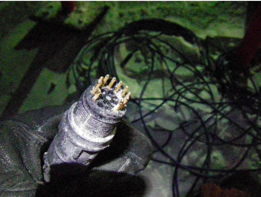
Photo 14: The plastic surrounding the pins on the connector of ND-HTS-175-32.5.
